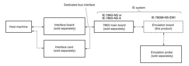
Figure 1-3. Basic Hardware Configuration (When IE-78K0-NS-A Is Used)
