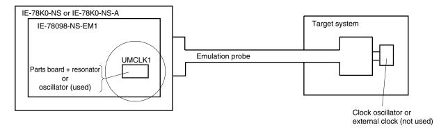
**Remark** The clock that is supplied by the resonator of the IE-78098-NS-EM1 (encircled in the figure) or the oscillator is used.
