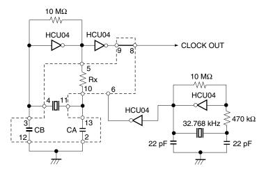
Remark The sections enclosed in broken lines indicate parts that are attached to the parts board.
