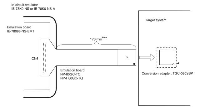
Note Distance when NP-80GC-TQ is used. When NP-H80GC-TQ is used, the distance is 370 mm.
