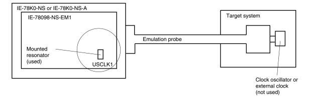
**Remark** The clock that is supplied by the resonator of the IE-78098-NS-EM1 (encircled in the figure) is used.
