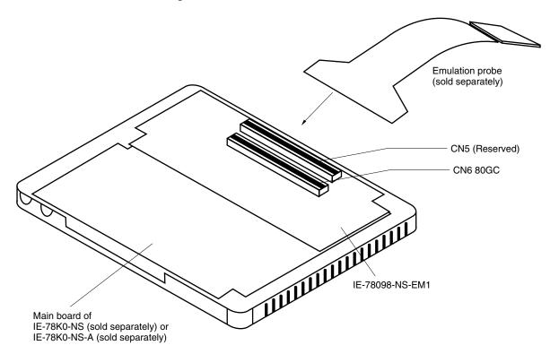
Figure 3-1. Connection of Emulation Probe
