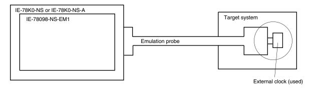
**Remark** The pulse that is supplied by the external clock on the target system (encircled in the figure) or the oscillator is used.
