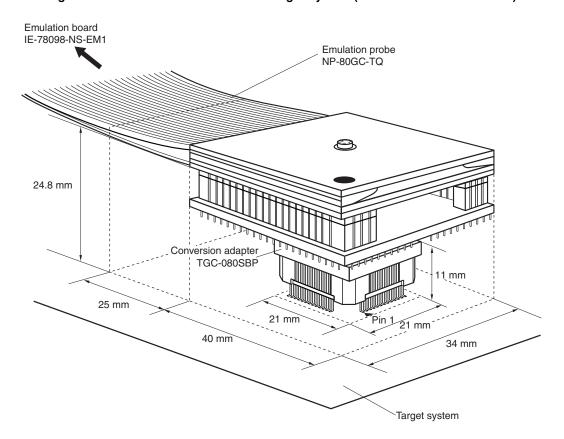
Figure B-2. Connection Conditions of Target System (When NP-80GC-TQ Is Used)
