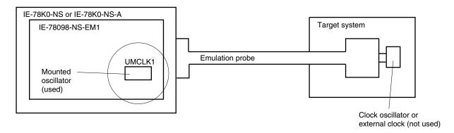
Remark The clock that is supplied by the oscillator of the IE-78098-NS-EM1 (encircled in the figure) is used.
